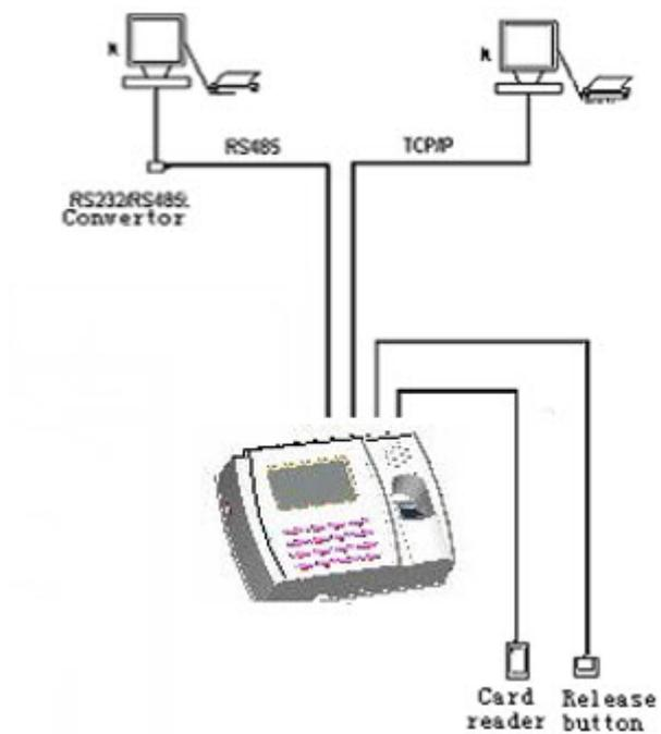
This device supports RS232 and TCP/IP connections to the PC.
