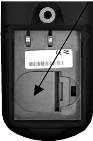
This battery does not have to be replaced until prompted by a warning message. If you see a transparent film insulating the backup battery, please remove it now.
