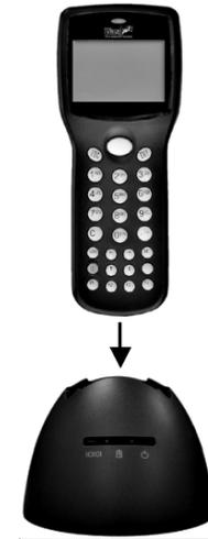
Place the WDT2200 in the cradle to begin the charging cycle. When the red LED turns green, the battery is fully charged. (Note: The LED on the cable itself is always green when powered and connected to a cradle.)
