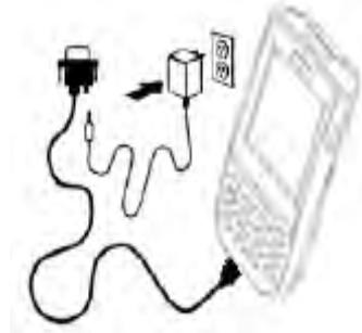
Or place the WPA206 into the Docking Station (first connect the power supply to the Docking Station).
