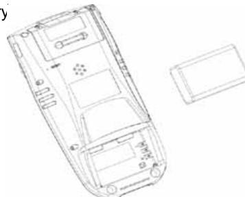
3. Position the battery pack and install the battery compartment door by using sylus screw driver.
