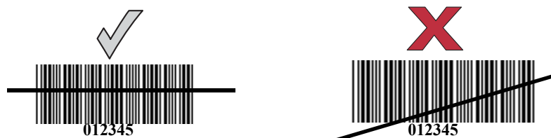
Figure 2-3. Acceptable and Incorrect Single-Line Aiming
