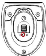
Insert the power supply to the DC Jack at bottom of the scanner. When charging, the scanner LED will flash RED. When the battery is fully charged, around 4 hours from completely empty battery, the LED stays on solid RED.
