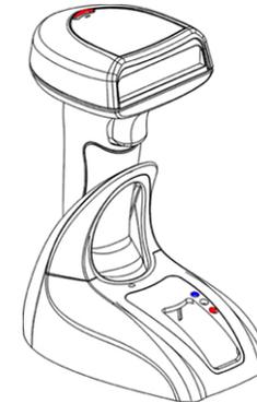
Place the scanner (with the battery inserted) on the base to charge your scanner. When charging, the scanner LED will flash RED. When the battery is fully charged, around 4 hours from completely empty battery, the LED stays on solid RED.
