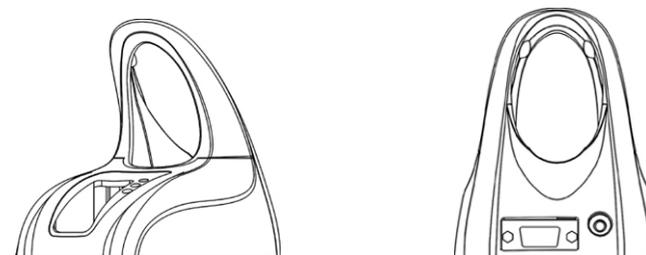
Connect the interface cable into the 15-pin connector at the back of the base. There are three types of cables available: RS232, Keyboard or USB.
