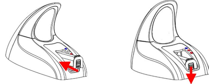
Insert the battery in front of the base to charge your battery with the power adaptor connected. When charging, the base charging LED will be RED. When the battery is fully charged, around 4 hours from completely empty battery, the LED will be solid GREEN.
