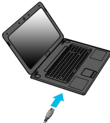
2. Connect the micro USB connector to the micro USB port at the bottom of the device.
