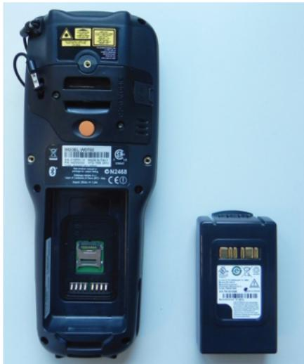
4. Insert the new battery pack into the slot (see [Install the Battery on page 7](#)).
