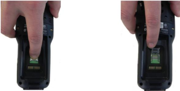
4. Insert the microSD card with the written part upward:
