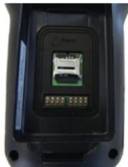
5. Lock the card into place by pushing the cardholder down and then shifting it downwards:
