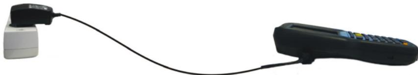
The Micro-USB port can also be used to charge the WDT92 battery pack from any self-powered USB hub or USB port on a computer.
