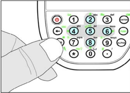
2. While holding the **TAB** key, insert the tip of the stylus into the reset hole on the back of the WPA1200 and press and hold the reset button until you see the splash logo screen appear and then release the **TAB** and reset buttons.
