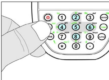
2. While holding the **Backspace** key, insert the tip of the stylus into the reset hole on the back of the WPA1200 and press and hold the reset button until you see the splash logo screen appear and then release the **Backspace** and reset buttons.
