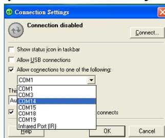
When you installed your Bluetooth dongle or setup your integrated Bluetooth, a COM port was selected. Select the same COM port here. If you are not sure which COM port was selected look in your BT dongle or integrated BT settings.
