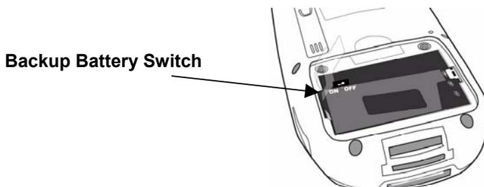
3. Position the battery pack, making sure the battery contacts are aligned with the contacts in the compartment and the battery is placed on top of the plastic tab, as shown in the following illustration.
