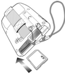
3. Push the card into the slot until you hear an audible system sound; this will signal that the card is already properly seated within the slot.
