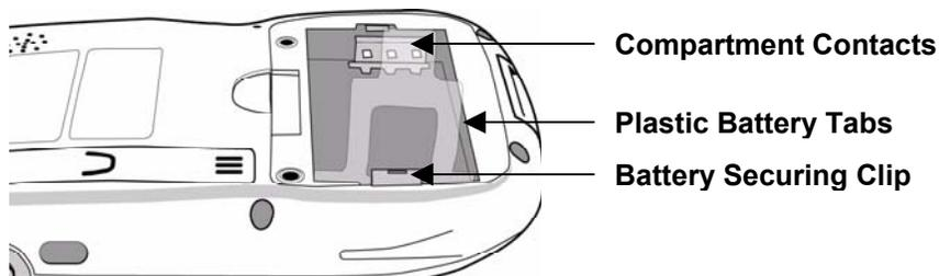
**Note:** The plastic battery tab makes it easy to remove the battery.
