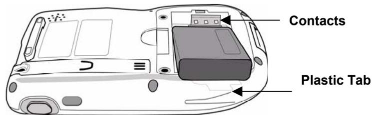
4. Slide the battery pack into the battery bay while simultaneously pulling the securing clip until the battery clicks into place.
