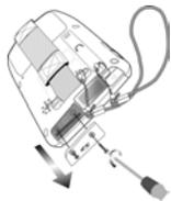
2. Insert the SD card with the notched corner as shown by the icon on the case.
