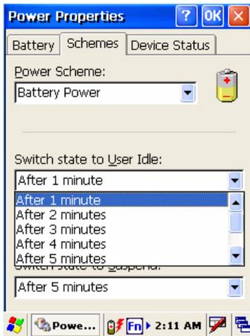
2. Tap the **Switch state to User Idle**, **Switch state to System Idle** or **Switch state to Suspend** option to select from a list of time periods. The available time periods are 1, 2, 5, 10, 15, 30 minutes and never.
