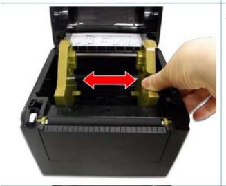
2. Separate the media holders to the label roll width.
