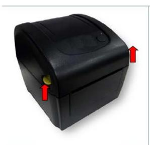
Open the printer top cover by pressing up the top cover open tabs located on each side of the printer.
