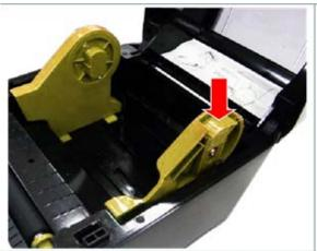
1. Please refer to section 3.2.2 to fix the media holders for installing the 1.5" adapters.
