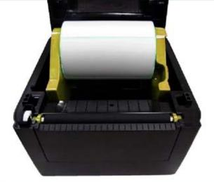
3. Place the roll between the holders and close them onto the core.
