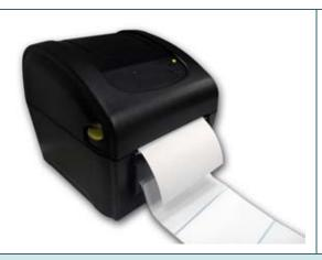
5. Printer is ready for peel-off mode. Print a label for test.
