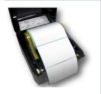
4. Place the label leading edge onto the platen roller. (printing side face up)
