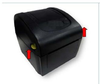
1. Open the printer top cover by pressing up the top cover open tabs located on each side of the printer.
