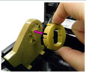
2. Press 1.5" adapters into both media holders for using 1.5: core media roll.
