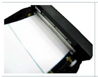
1. Please refer to section 3.2.1 to load the media. Lead the paper through the cutter paper opening.
