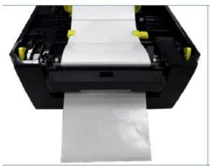
6. Close the peel-off cover and printer cover. Printer is ready for peel-off mode.
