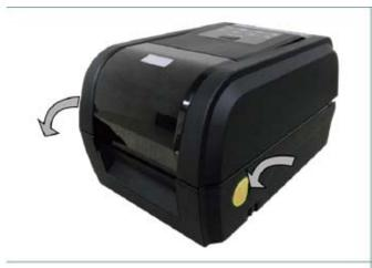
1. Open the printer's top cover by pulling the top cover open levers located on each side of the printer and lifting the top cover to the maximum open angle.
