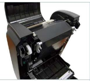
7. Stick the ribbon onto the ribbon rewind paper core.
