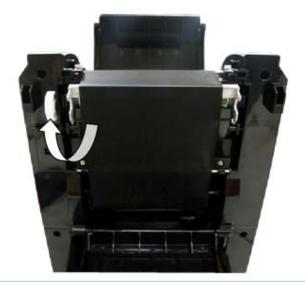
8. Turn the ribbon rewind gear until the ribbon plastic leader is thoroughly wound. Close the ribbon access cover and the top cover.
