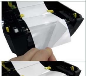
5. Open the peel-off cover. Feed the liner into peel-off cover slot.
