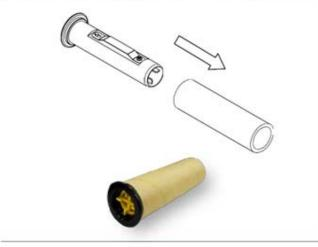
3. Insert the rewind spindle into the paper core.
