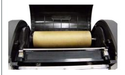
5. Insert the ribbon spindle into the ribbon core.
