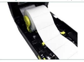
1. Please refer to section 3.3.1 to feed the paper, printing side face up, through the paper guide and pass over the platen.
