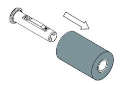
6. Install the ribbon right side onto the supply hub first then align the notches on the left side and mount onto the spokes.
