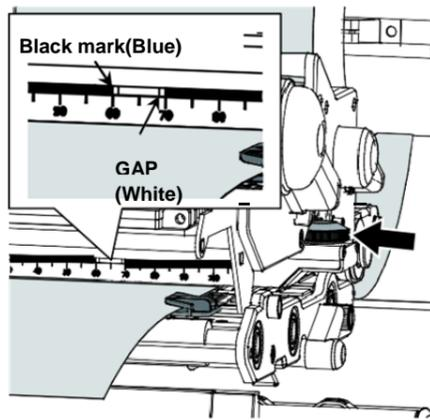
(4) Adjust the rear label guide (green) to fit the label width.
