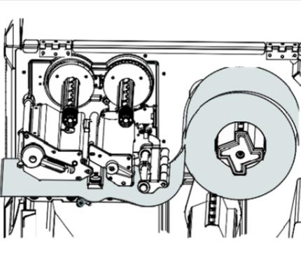
(1) Open the printer right side cover. Place the roll of media on the label supply spindle.
