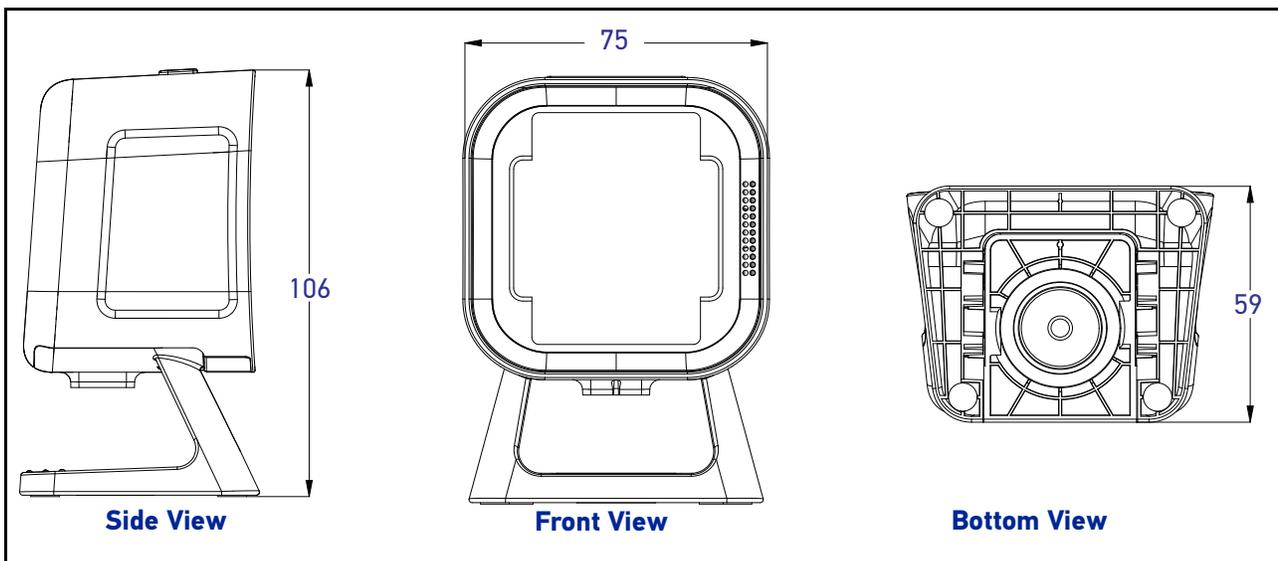
Figure 7. Dimensions for Scanner with L Bracket / Wall Mount
