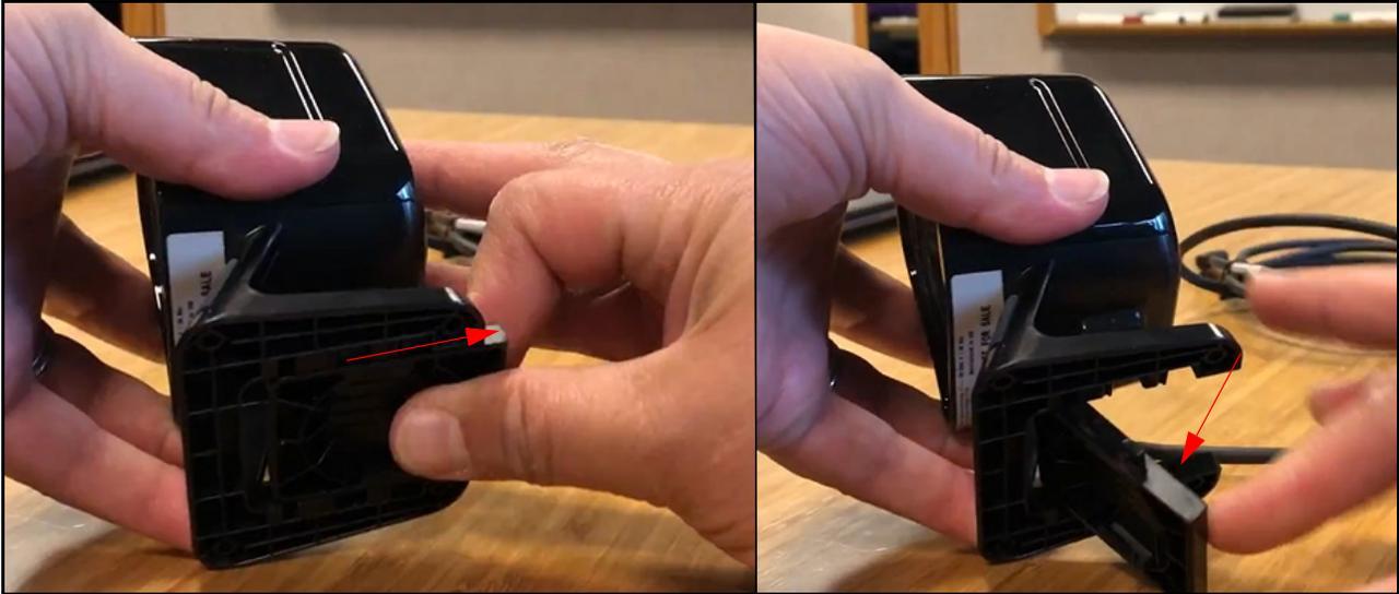
6. Plug the interface cable straight in and ensure it clicks securely into place, then push the door back up and slide it forward to close it again.
